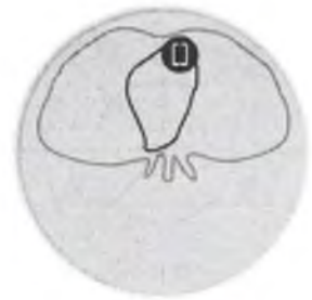
Figure 5 - T310d 5GHz Elevation Antenna Patterns
